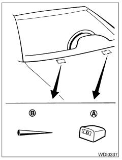
If you wax the surface of the hood, be careful not to let wax get into the washer nozzle (A). This may cause clogging or improper windshield washer operation. If wax gets into the nozzle, remove it with a needle or small pin (B).
