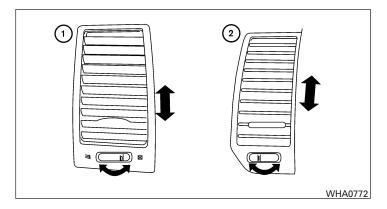
Adjust air flow direction for the driver's and passenger's side (1), and center (2) ventilators by moving the ventilator slide and/or ventilator assemblies.
