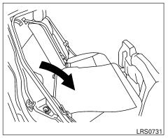
Fold down seatbacks. See "Interior trunk access (if so equipped)" earlier in this section.
