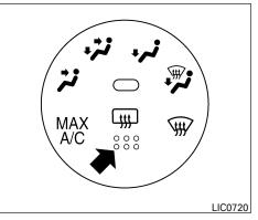
To defrost the rear window glass and outside mirrors (if so equipped), start the engine and push the rear window defroster switch on. The rear window defroster indicator light on the switch comes on. Push the switch again to turn the defroster off.
