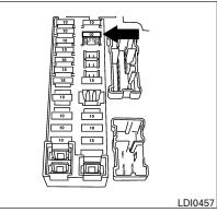
If a type A fuse is used to replace a type B fuse, the type A fuse will not be level with the fuse pocket as shown in the illustration. This will not affect the performance of the fuse. Make sure the fuse is installed in the fuse box securely.
