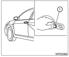
All doors will be locked automatically unless one of the following operations is performed within 60 seconds after pushing the request switch.
