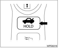
Releasing the trunk lid (if so equipped)
