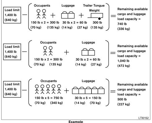
Steps for determining correct load limit
