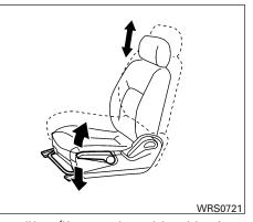
Seat lifter (if so equipped for driver's seat)
