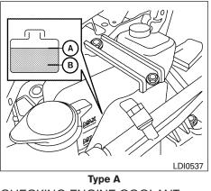
CHECKING ENGINE COOLANT LEVEL
