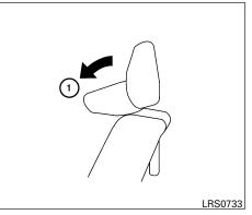
2. Fold down the rear head restraint. Pull the head restraint forward and rotate until it clicks into the locked position ①.
