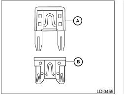
Two types of fuses are used. Type (A) is used in the fuse boxes in the engine compartment. Type (B) is used in the passenger compartment fuse box.
