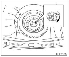
2. To remove the jack, turn the jack screw counterclockwise and lift out.
